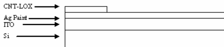
Figure 5.1. Schematic drawing of CNT-LOX on Si/ITO electrode.
